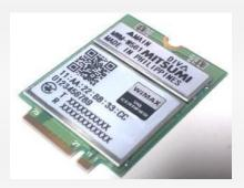
The MWM-W56x series supports all M.2(NGFF) features to optimize performance, power consumption, and usability. The module has advanced features such as TX diversity and high throughput in uplink-downlink.
