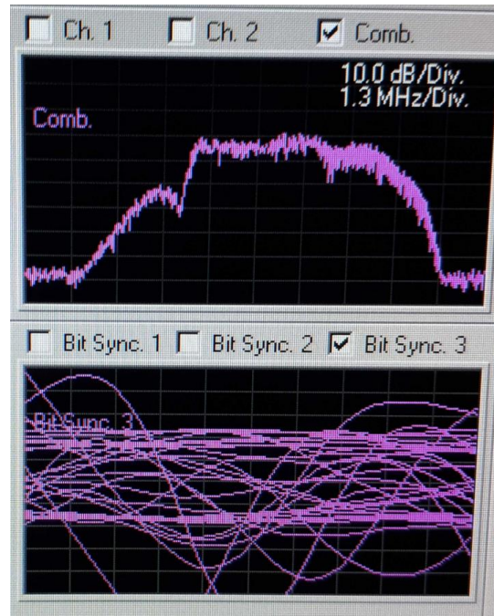
Figure 29: Reception condition of the telemetry station of the airplane at 300Km based on the spacing of 5MHz between services.
