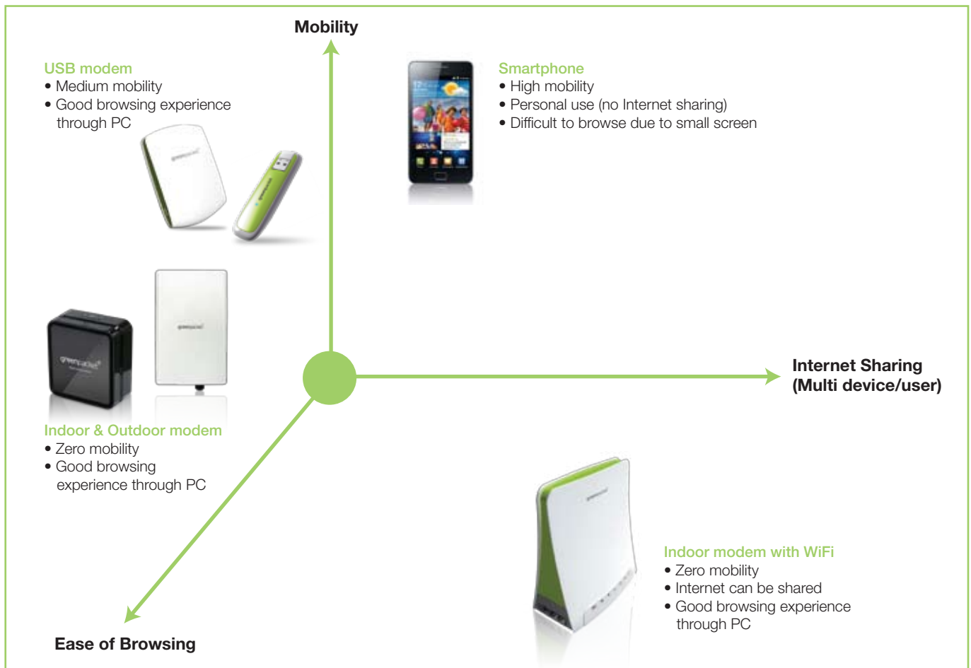
Figure 7: Characteristics of WiMAX Devices from the Aspect of Mobility, Internet Sharing and Ease of Browsing
