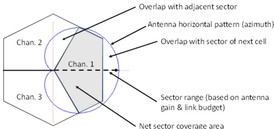
Figure 7: Sector or Channel Coverage for 15 dBi BS Sector Antenna
