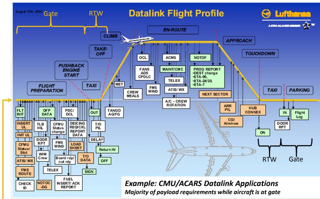
Figure 9: ACARS Datalink Applications
