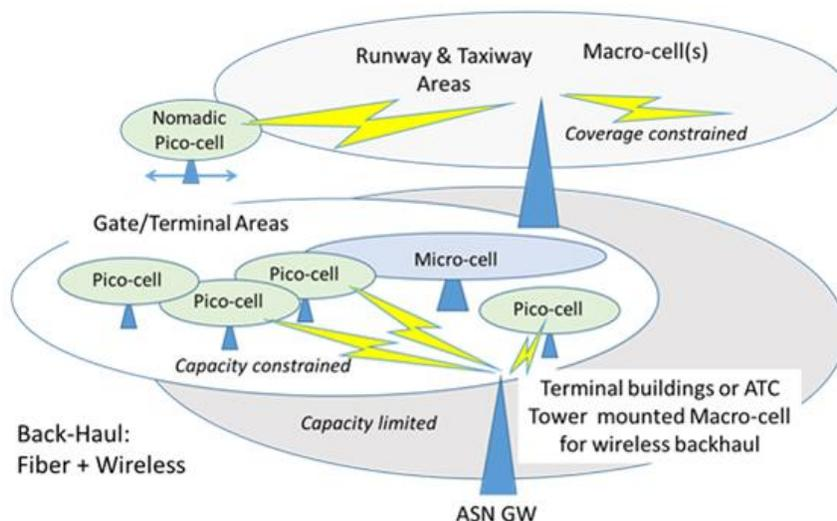
Figure 6: A large airport has varied BS requirements for coverage and capacity
