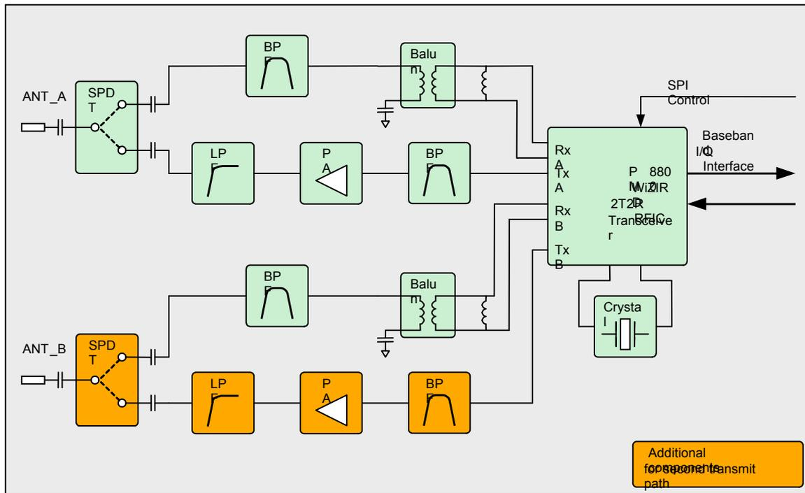
The additional size required for the additional components is approximately 50 mm<sup>2</sup> (this will vary depending on the components chosen). In the future, this could even be smaller, as integrated front-end modules (FEM) are used. Note that some FEM vendors are planning integrated dual-FEM designs in a single package. This process would further reduce the impact of the second transmitter.
