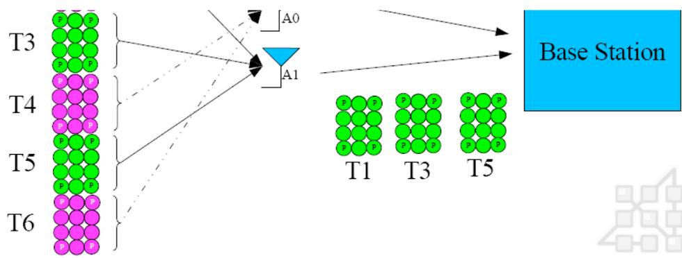
Because coding is performed on a slot-by-slot basis, the diversity introduced by TSD on the tiles will be exploited by the convolutional encoder to reduce the error probability. The exact order of diversity is directly a function of the coding order. Furthermore, a TSD scheme can be further enhanced by the use of MRC at the base station.
