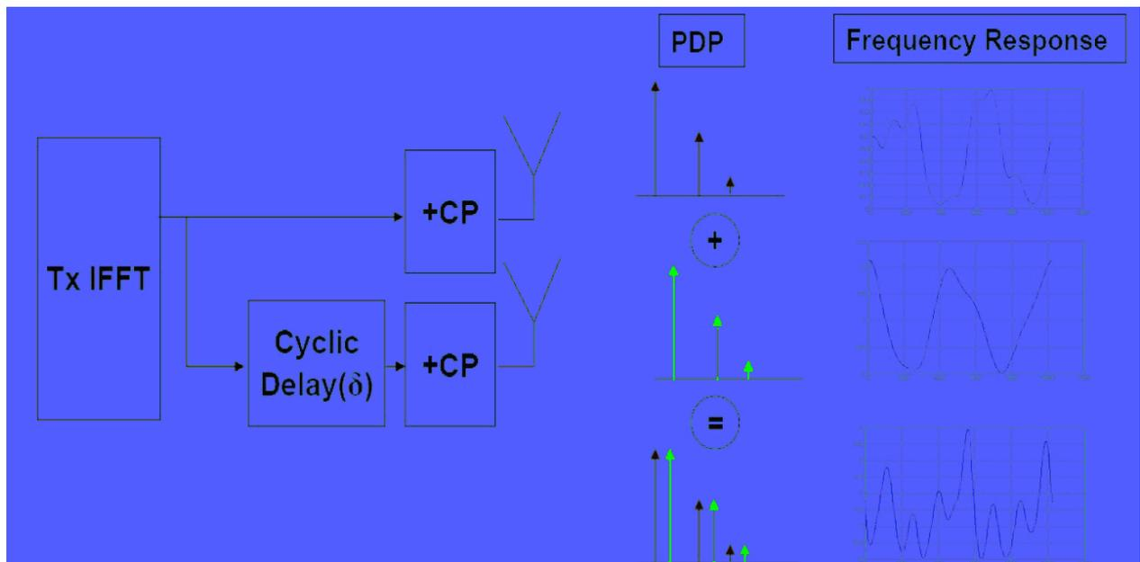
It is a simple way of adding diversity to a system, and performs well in fading environments [4].
