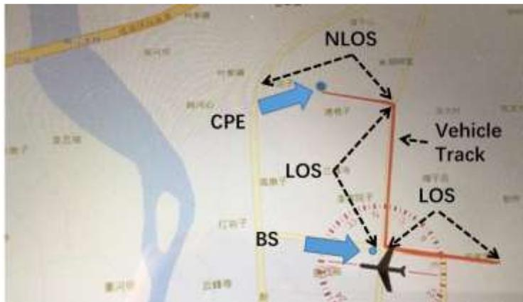
Figure 13. Vehicle surveillance test (c)
