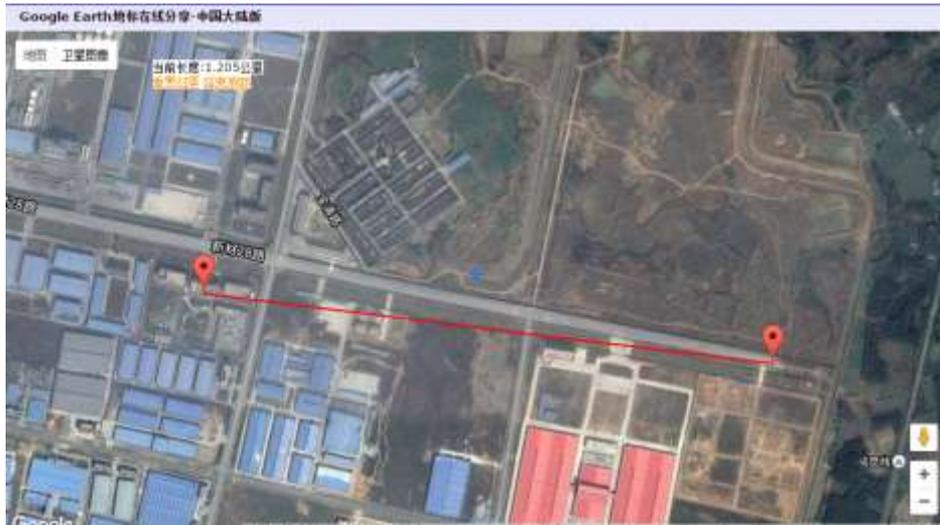
Figure 4. Position relation between BTS and CPEs.
